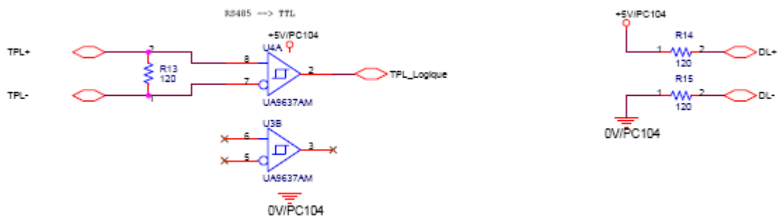
Figure 1. Diagram of the electronic of reception of the trig Balise and the Down Link
